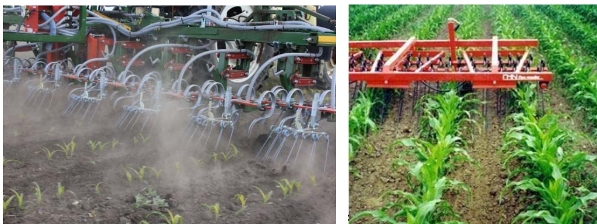
Row cultivator with seeding equipment (left) and harrow with seed box (not in picture) Photos: Poul Henning Pedersen, VFL and CMN Maskintec A/S
